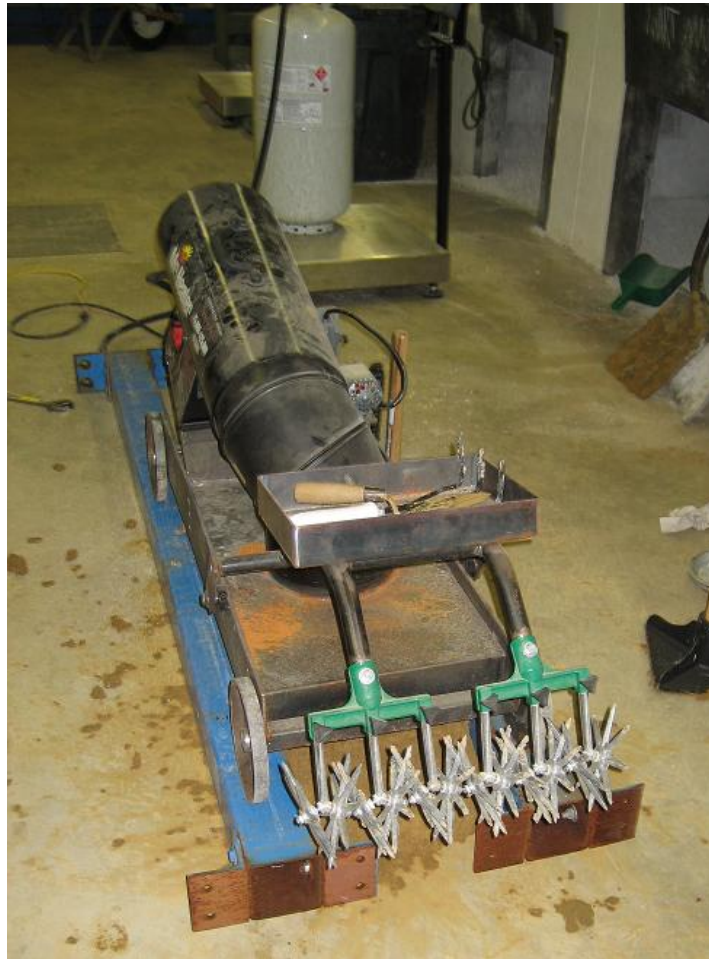
Figure 10. PRO-SD in operation over a 4 inch depth soil sample.
