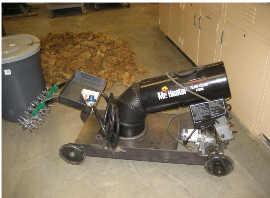
Figure 4: PRO-SD Laboratory Scale Propane Soil Drying Device
